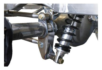
**Step 9:** Attach the Shock Crossmember to the top of the Coilovers and mark on the frame where it will land on both the Drivers and Passengers Side.
