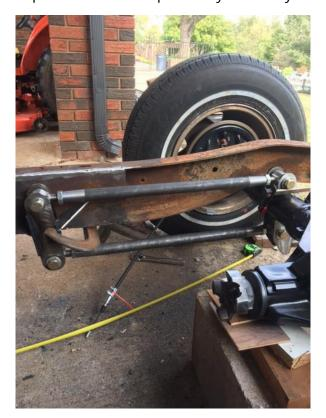
**Step 8:** Take the rear coil-overs and bolt them onto the rear end brackets that you have tacked in place in Step 3.
