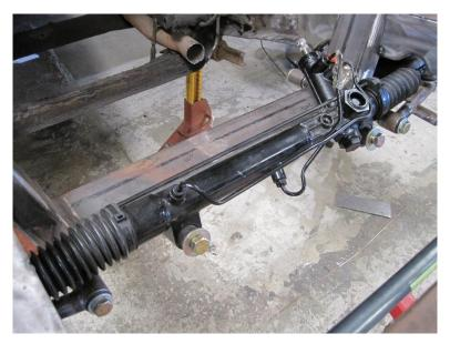
Start by holding the Spindles as close to straight as possible. Thread the Outer tie Rod End IN or OUT until it lines up with the Spindle Steering Arm. Do not tighten yet as this will need to come back off for alignment. Adjust both Driver's and Passenger's Outer Tie Rod Ends evenly.
