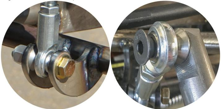
Mount the Sway Bar Bushing/Bracket to the Sway Bar. Hold the Sway Bar up to the underside of your frame rails. The Heim link should be straight up & down while the Sway Bar is level with the Lower A-Arm. Some applications will allow you to mount the Bushing/Bracket directly to the underside of the Frame Rail. Other applications will need to utilize the supplied Sway Bar Bracket.
