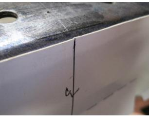
**STEP 2**Fit the boxing plate into the frame and tack it in place
