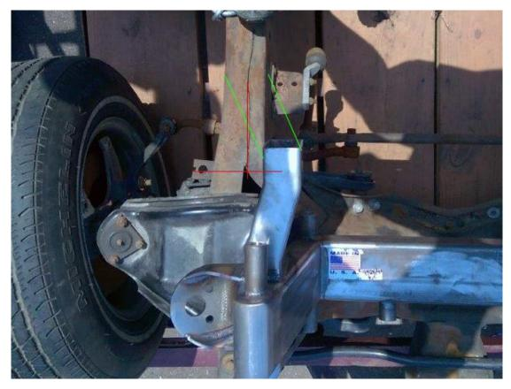
**STEP 3**Mock Up the crossmember in position. You will have to graph your stock frame rails to the frame rail sections that we have welded to the IFS crossmember.
