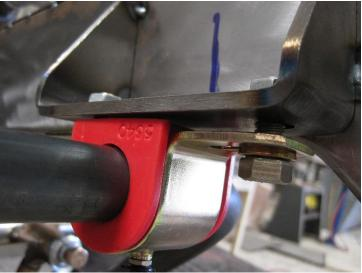
**STEP 5**Adjust the heim to get the Sway Bar level with the Lower A-Arm at Ride Height.
