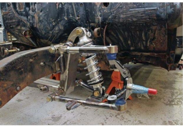
15. Once the spindles are in place the disc brake caliper brackets are bolted on.
