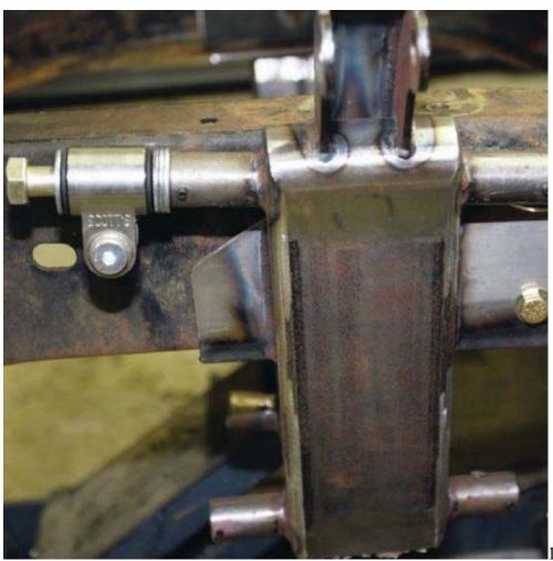
11. When adjusting caster and camber the number of spacers needed will increase or decrease as the clevises screw into or out of the upper A-frames. Once the adjustments are made, the attachment bolts are secured with setscrews.
