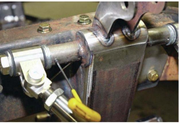
12. The lower A-frames include mounts for the Aldan coilovers (or air bags as well as the sway bar links if ordered).
