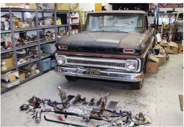
3. The day before disassembly begins every fastener you can reach should be sprayed with penetrating oil. This is so they will come apart easily.
