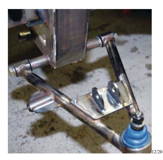
13. Attaching the spindles is easy enough; however, the included thick washers must be used under the nuts.
