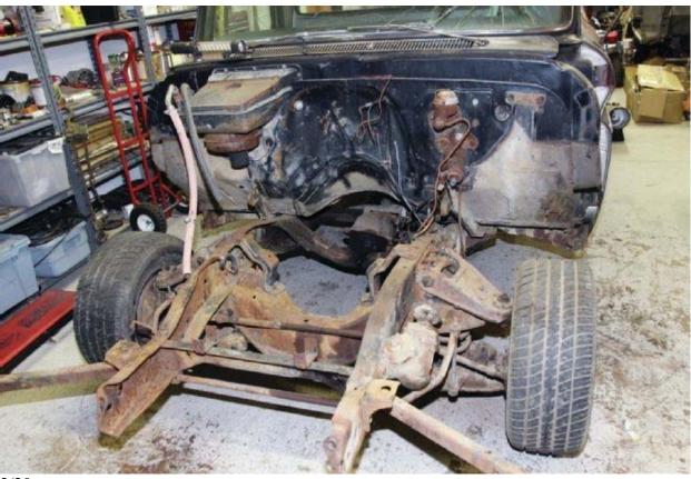
4. With the front sheetmetal removed, unbolt the entire front suspension and lower it to the floor.
