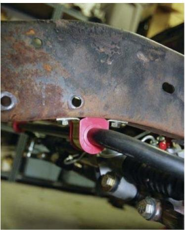
19. Urethane bushings (if purchased) are used in the sway bar's frame mounts and pairs of heim
