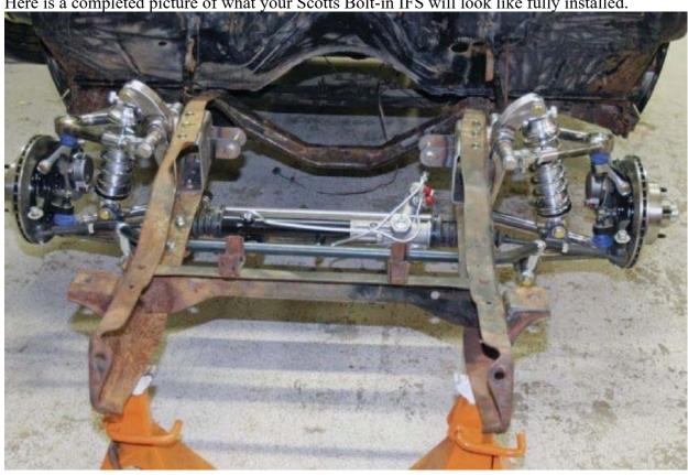
2. Scott's bolt-in front suspension system comes with everything required, including all the fasteners in labeled bags.
