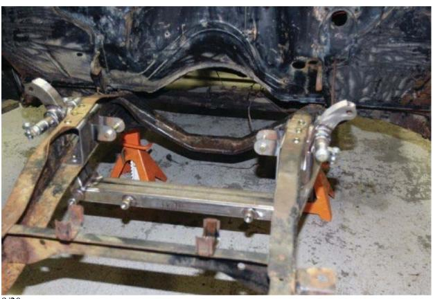
10. On each side, the upper A-frame attaches to the crossmember with a stainless steel clevis. Note the spacers between the clevis and the crossmember.
