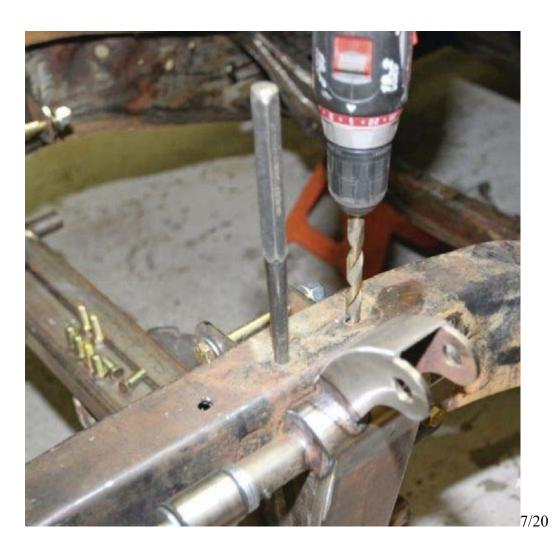
8. Like the original, the Scott's crossmember bolts to the tops, sides, and bottoms of the framerails.
