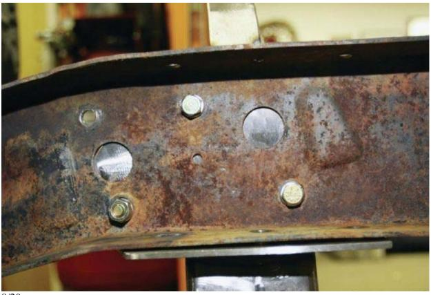
\*\*NOTE\*\* If you are installing a Scott's 73-87 C-10 Bolt-in IFS the very top hole will need to be drilled on your frame do to the stock hole location and where our crossmember sits, simply locate and drill a 9/16 hole. \*\*
