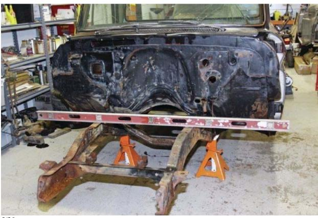
6. Use a floor jack to raise the new crossmember into position. The inner frame reinforcements (if you purchased Motor Mounts) have engine mounts already in place (there are a variety of block brackets available to accommodate various engines).
