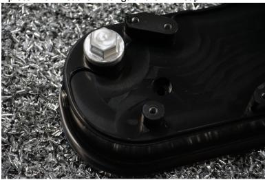
Remove stock valve covers. Next you will need to install the Stand-Offs directly onto the heads included with your Scott's Hotrods Valve Covers. Install a stock replacement O-Ring Gasket to the Lower Half of the Scott's Valve 'n Coil Covers. Bolt the Valve Cover to the Stand Offs using supplied hardware.
