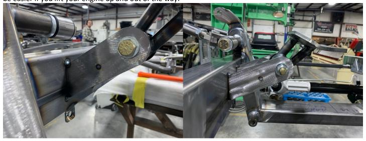
Step 6: Lower your motor back down and slide the bushing side of the mount in between your tacked D-Tabs. Be sure you can slide the long bolts through. Sometimes they need a little encouragement from a mallet. This is why the Bolts holding the mount to block should not be fully torqued at this time.
