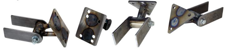
Step 1: Bolt the Motor Mounts to your block with your hardware. Do not torque them down at this time. Simply snug them up, but not too tight so you can wiggle them into place if needed. The Driver's Side is labeled with a "D" and the Passenger Side with a "P."
